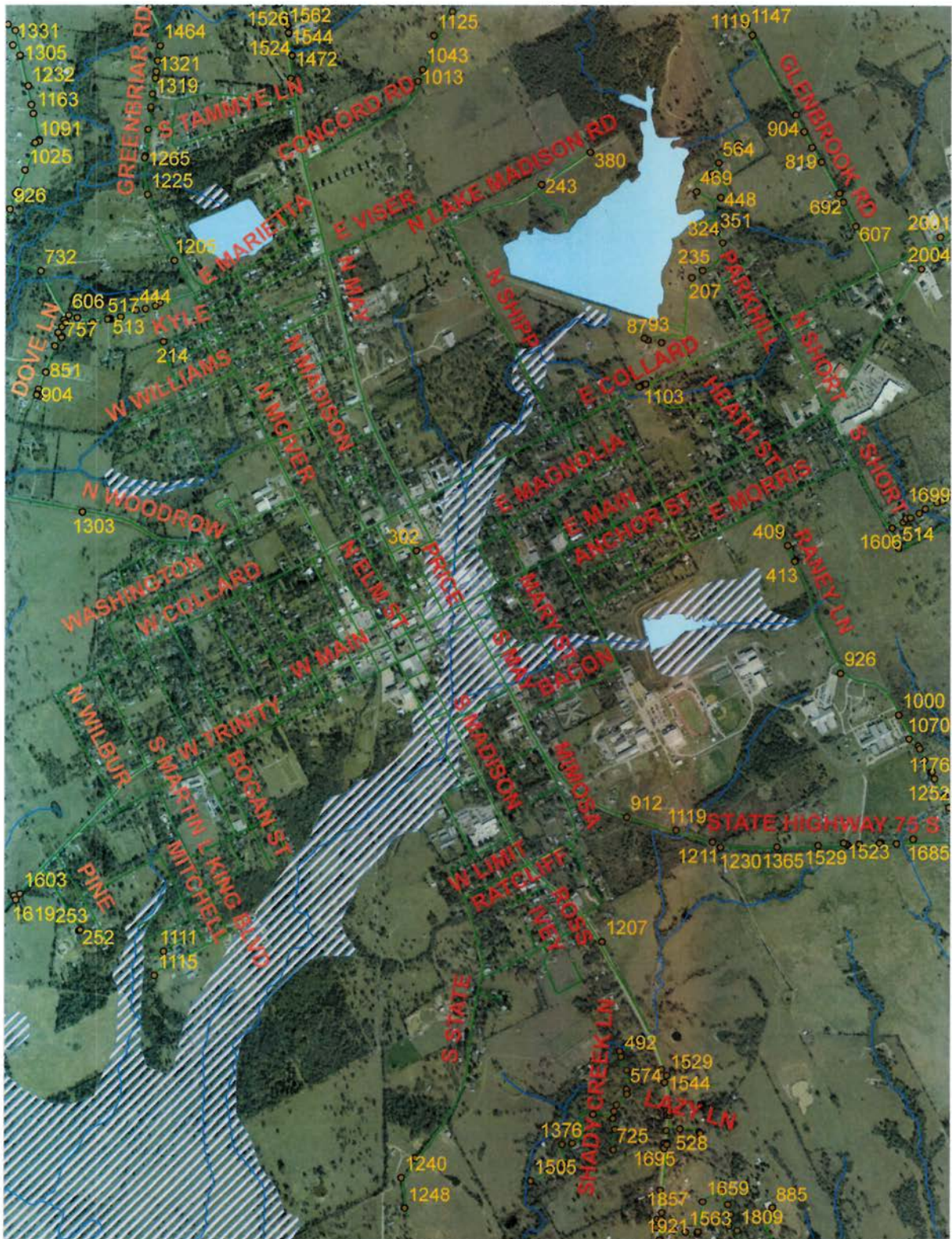
Figure 14-1. Possible Inundation Areas for Town Branch Dams and Crescent Lake Dam
